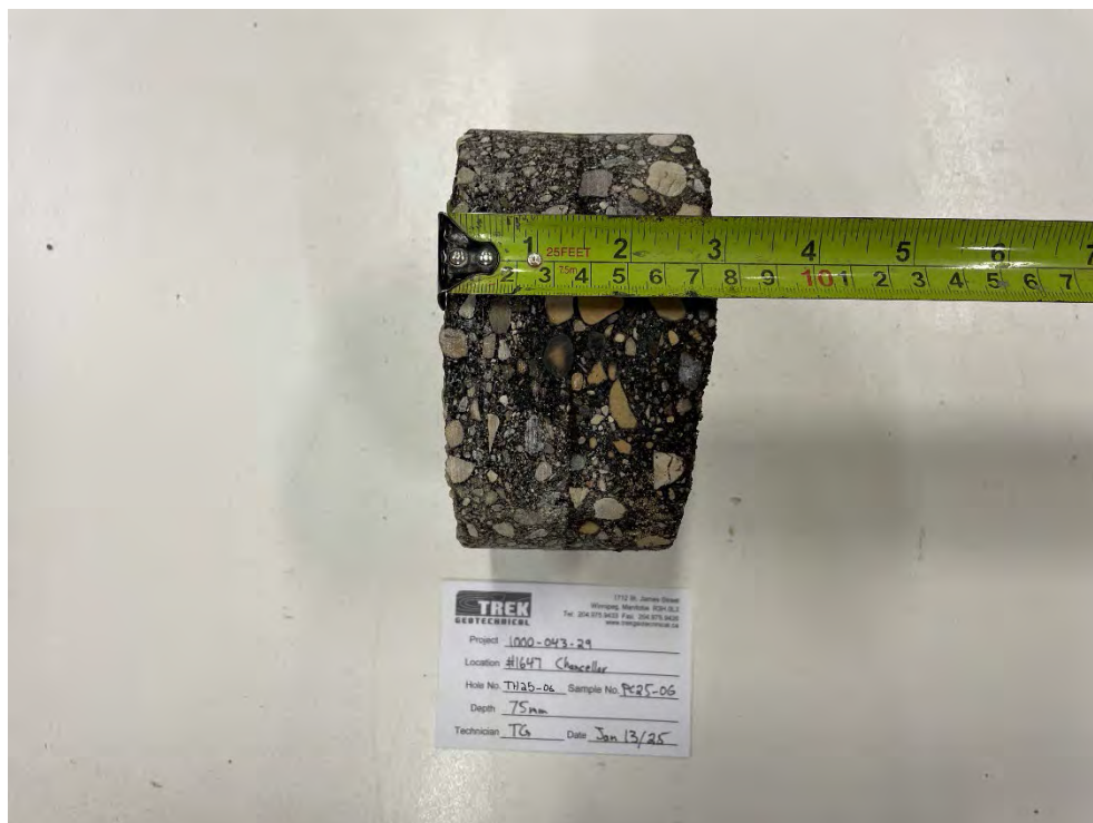
Photo 4: Pavement Core Sample at TH25-06
