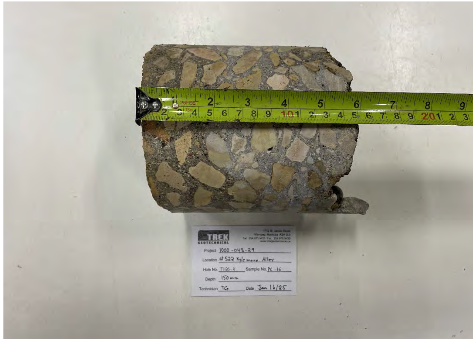
Photo 1: Pavement Core Sample at TH25-16
