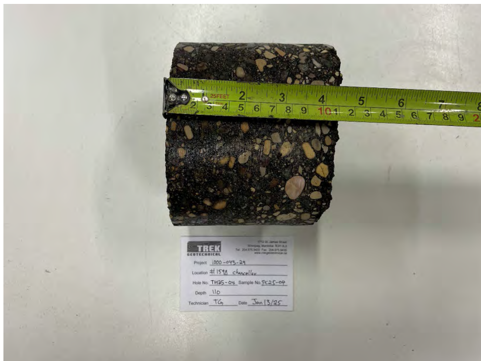
Photo 2: Pavement Core Sample at TH25-04
