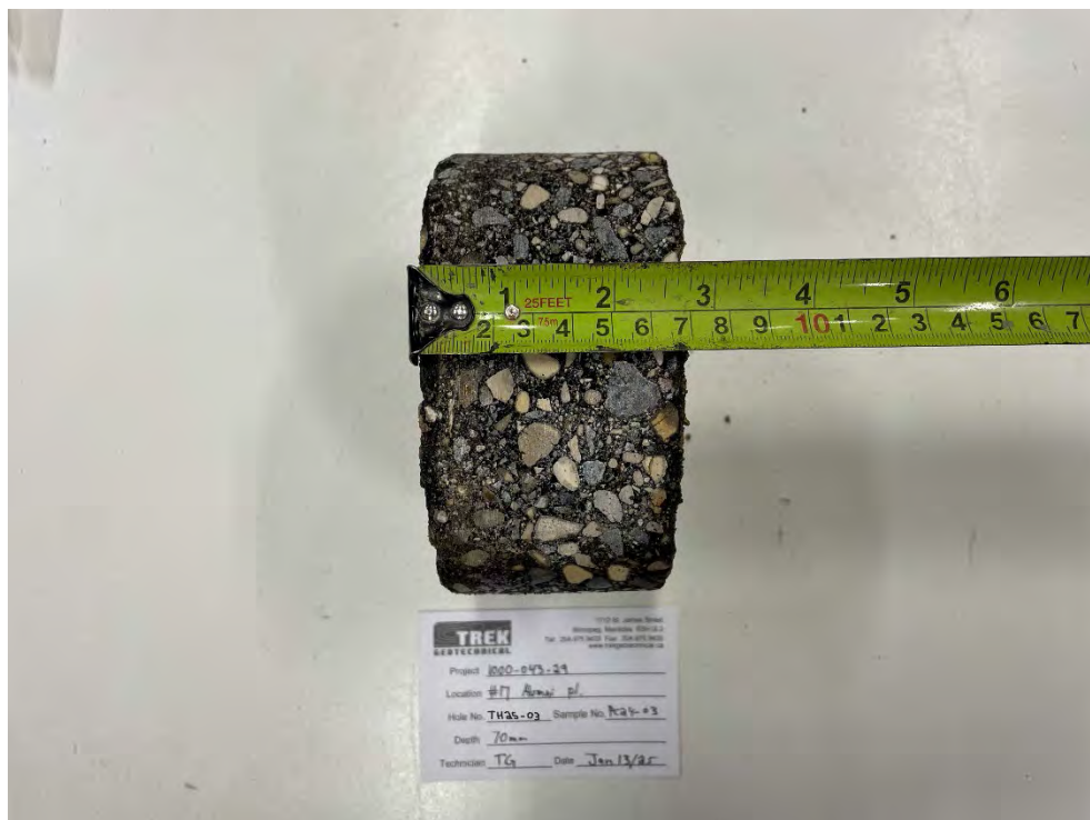
Photo 2: Pavement Core Sample at TH25-03
