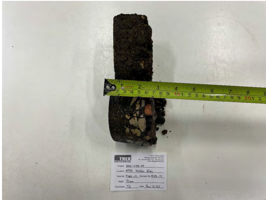
Photo 1: Pavement Core Sample at TH25-17
