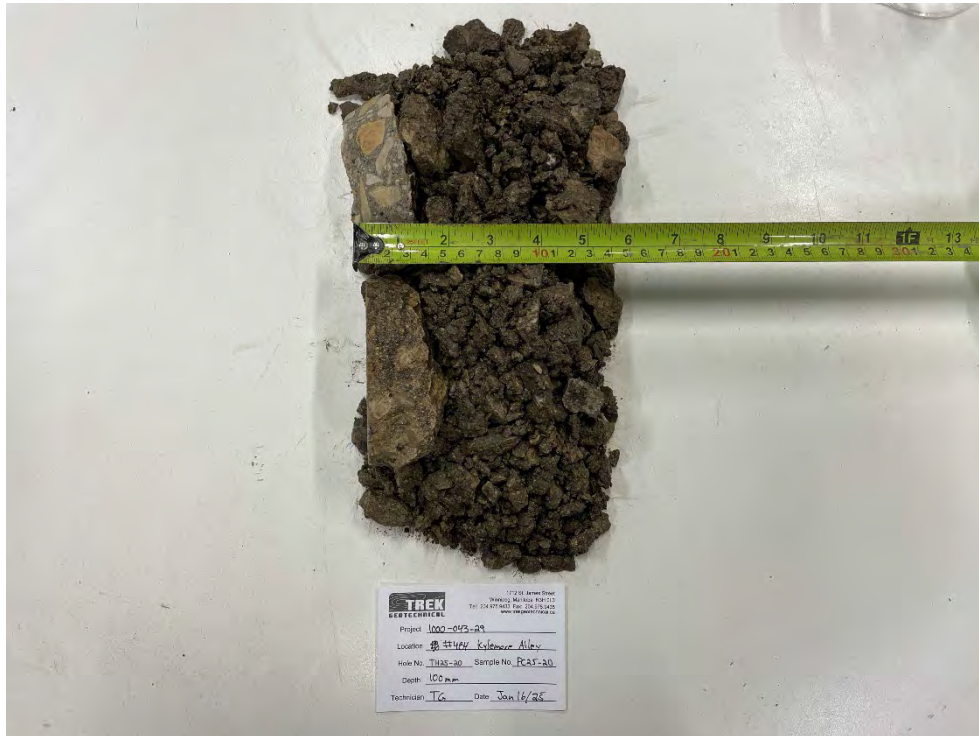
Photo 3: Pavement Core Sample at TH25-20
