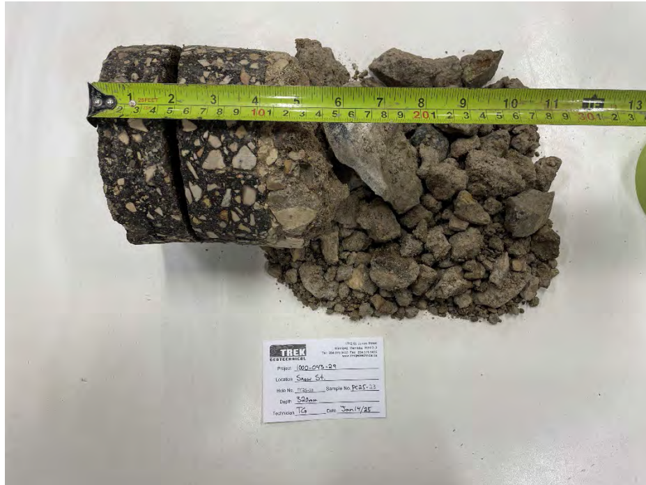
Photo 1: Pavement Core Sample at PC25-23
