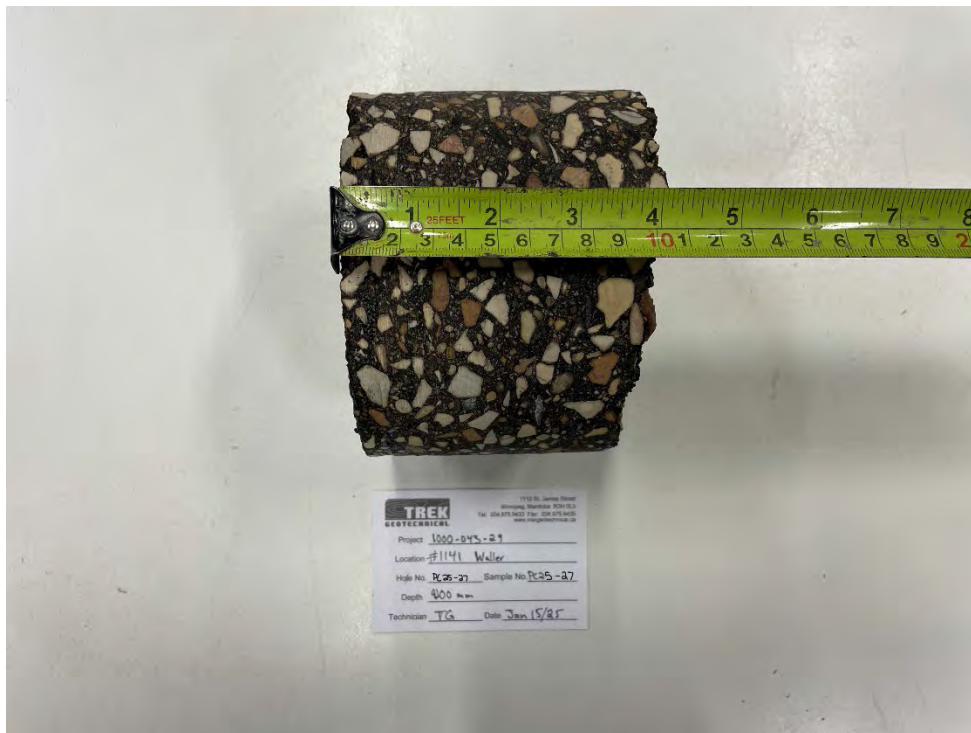
Photo 2: Pavement Core Sample at PC25-27
